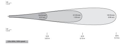
**PHI Coverage Guidelines** Ceiling **Max Coverage Max Coverage Recommended Size** 5 inch PHI (ft²) 9 inch PHI (ft²) Height (ft) (PHI, Nozzle) ~10 960 5200 5 inch PHI, Short ~15 640 3470 5 inch PHI, Short ~25 380 2080 9 inch PHI, Standard
