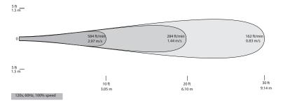
**PHI Coverage Guidelines** Ceiling **Max Coverage Max Coverage Recommended Size** 5 inch PHI (ft²) 9 inch PHI (ft²) Height (ft) (PHI, Nozzle) ~10 5200 960 5 inch PHI, Short ~15 640 3470 5 inch PHI, Short ~25 380 2080 9 inch PHI, Standard
