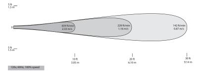
**PHI Coverage Guidelines** Ceiling **Max Coverage Max Coverage Recommended Size** 5 inch PHI (ft²) Height (ft) 9 inch PHI (ft²) (PHI, Nozzle) ~10 960 5200 5 inch PHI, Short ~15 640 3470 5 inch PHI, Short ~25 380 2080 9 inch PHI, Standard
