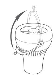
The Air Pear system is designed to hang vertically and freely 12-to-18 inches, or as close as possible, from the ceiling on professionally installed hardware, for models 10/15/25, capable of supporting a minimum of five times the weight of the Air Pear unit, 60 lb. (27 kg.). Example - 1/4" (7 mm) diameter steel bolt is rated at 60 lb. (27 kg.) load.
