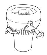
2 Swing the bail to the vertical position and retighten the two Torx screws.
