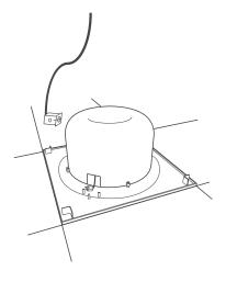
6 Plug the Suspended Series power cord into the receptacle. Using the supplied thumbscrews, fasten the j-box to the air intake grill through the indicated holes as shown (wiring to j-box omitted for clarity).
