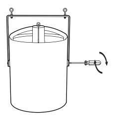
**3** The Q Series system is designed to hang vertically and freely 12-to-18 inches, or as close as possible, from the ceiling on professionally installed hardware capable of supporting a minimum of five times the weight of the Q Series unit, 60 lb. (27 kg.). Example - 1/4" (7 mm) diameter steel bolt is rated at 60 lb. (27 kg.) load.
