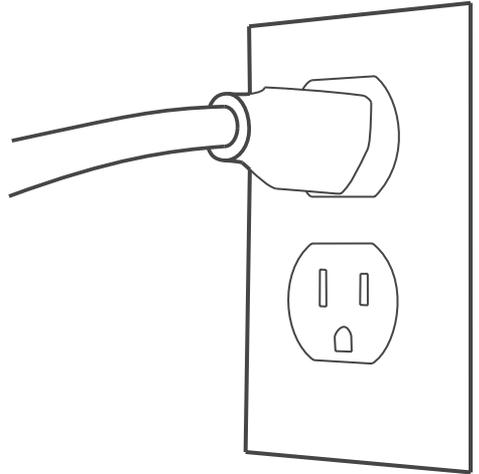
**6** NOTE: SECURE the power cord to the ceiling structure as added security. The cord will act as a safety leash and by securing it the possibility of the plug accidentally coming out of the outlet in the future is greatly reduced. A 50 lb. (20 kg.) rated Zip-Tie or mechanics wire are examples of methods of securing the power cord.
