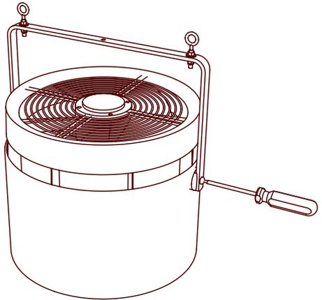
**3** The Onyx Series system is designed to hang vertically and freely 12-to-18 inches, or as close as possible, from the ceiling on professionally installed hardware, for models 10/15/25, capable of supporting a minimum of five times the weight of the Onyx Series unit, 60 lb. (27 kg.). Example - 1/4" (7 mm) diameter steel bolt is rated at 60 lb. (27 kg.) load.
